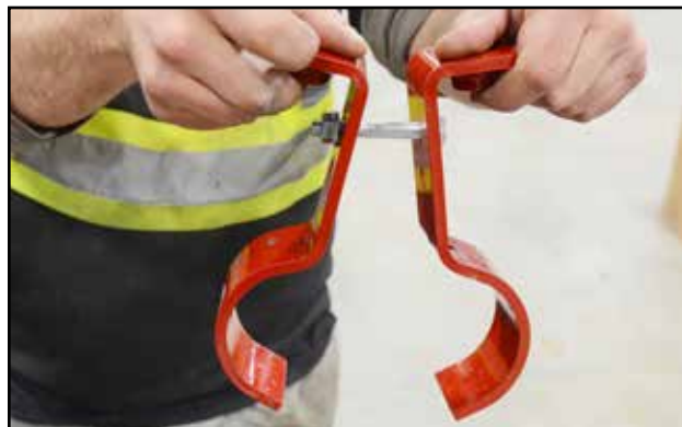
Fig 45 - 2 inch bolt joining the brackets
