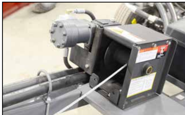
Fig 15 - Hydraulic winch for tube lift
