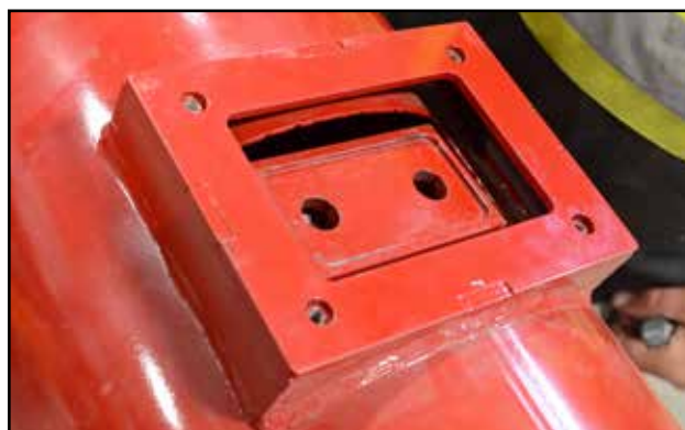
Fig 46 - Hanger bearing with Spacer Cover Plate
