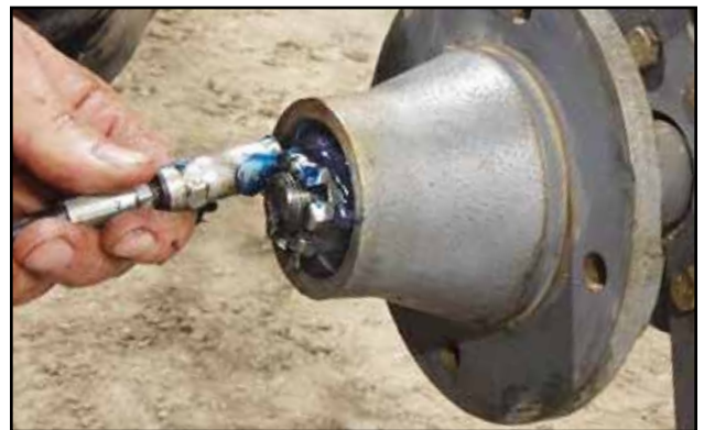
Fig 39 - Fill hub with grease
