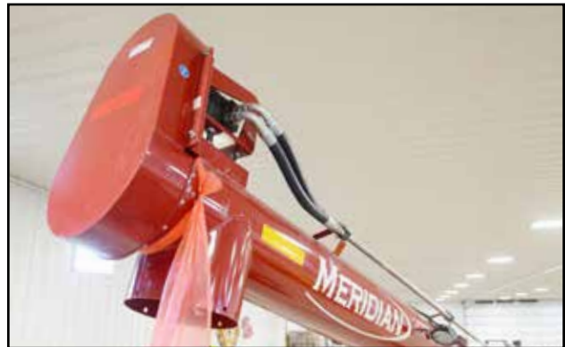
Fig 12 - Hydraulic drive for auger flighting
